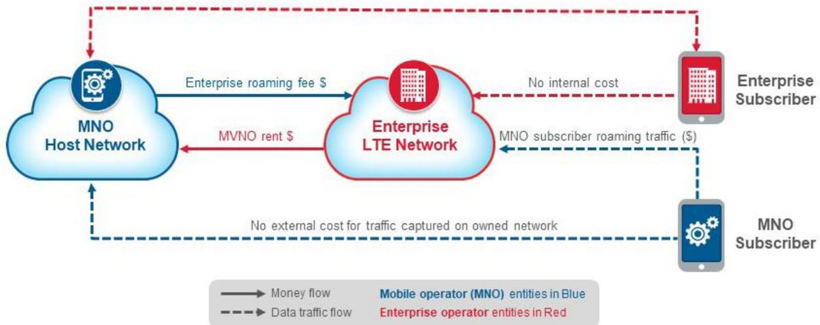
Figure 1 – MNO Managed Enterprise LTE Solution
